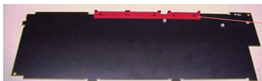
Figure 4 Completed replacement panel P/N 06050-20003. Now Ready for use in the instrument.
